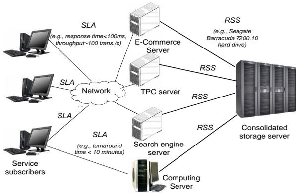
Fig. 1. There are three tiers in a typical system architecture involving consolidated storage service: service subscribers, application servers, and storage server. While the SLA-like performance interface describing bounds on response time and throughput is suitable between service subscribers and application servers, a different performance interface is needed between application servers and storage server, such as the reference storage system (RSS) proposed in this paper.
