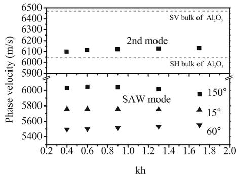
**FIGURE 7** Phase velocities as a function of the normalized film thickness  $kh$ . The dotted lines from the bottom to top represent  $v_{SH}$  and  $v_{SV}$  of  $Al_2O_3(11\bar{2}0)$  at  $0^\circ$  propagation angle, respectively
