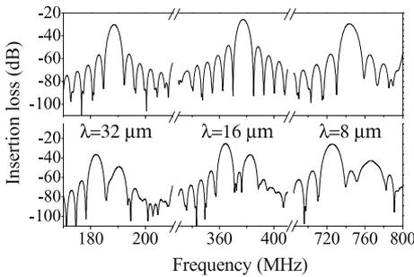
**FIGURE 4** The frequency response of the devices at different wavelengths. The *upper panel* is for the SAW devices propagating at  $150^\circ$ ; the *lower panel* is for the SAW devices propagating at  $0^\circ$
