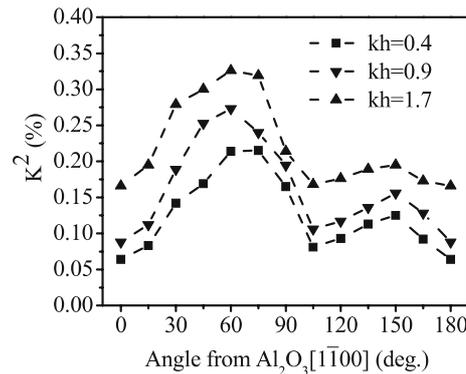
**FIGURE 6** Electromechanical coupling coefficients of the SAW as a function of the propagation angle
