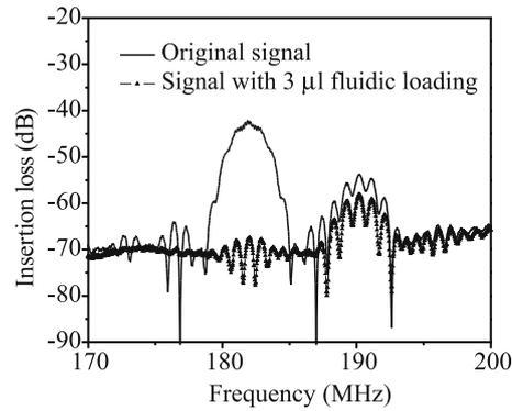
**FIGURE 8** Damping of the SAW and SH mode under liquid loading at wavelength  $\lambda = 32 \mu m$
