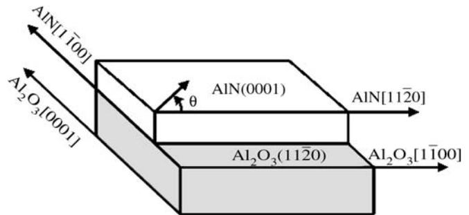
**FIGURE 3** Epitaxial growth relationships of the  $\text{AlN}(0001)/\text{Al}_2\text{O}_3(11\bar{2}0)$  structure. The angle  $\theta$  represents the SAW propagation angle measured from the  $\text{Al}_2\text{O}_3[1\bar{1}00]$  reference
