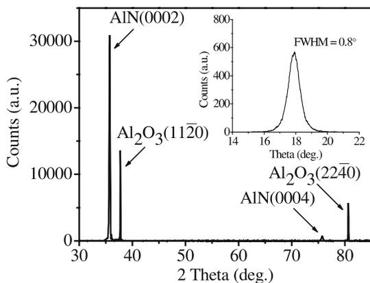
**FIGURE 1** XRD scan of the  $\text{AlN}(0001)/\text{Al}_2\text{O}_3(11\bar{2}0)$  structure (film thickness: 2  $\mu\text{m}$ ). Inset is the  $\text{AlN}(0002)$  rocking curve with a FWHM of  $0.8^\circ$
