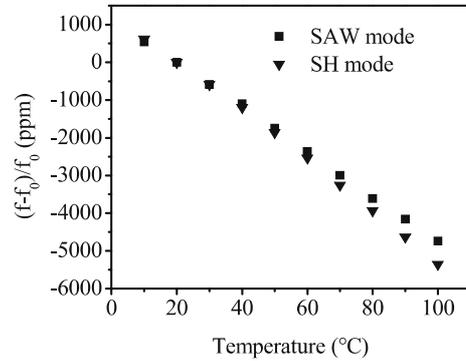
**FIGURE 9** Fractional frequency change as a function of temperature for the SAW and SH mode at a normalized film thickness of  $kh = 0.4$
