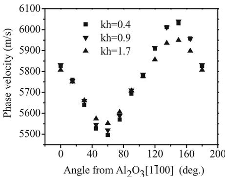
**FIGURE 5** Phase velocities of the SAW as a function of the propagation angle
