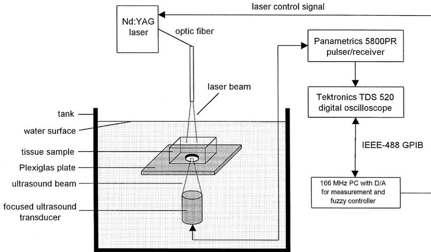
Fig. 1. Experiment set-up for ultrasound-guide fuzzy control of laser tissue coagulation.
