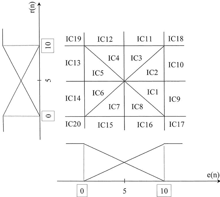
Fig. 2. Division of the input space into 20 regions for analytical structure derivation of the fuzzy controller. Input fuzzy sets for the input variables are also shown.
