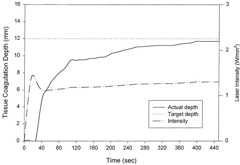
Fig. 3. One experimental result: progress of ultrasonically measured coagulation depth and the corresponding laser intensity.
