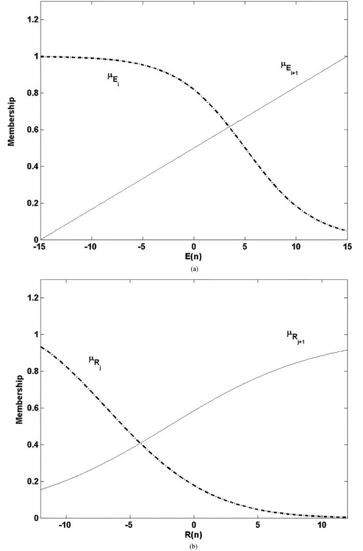
Fig. 2. Two example fuzzy sets for  $E(n)$  (a) for  $\mu_{E_i}$  and  $\mu_{E_{i+1}}$ . Two example fuzzy sets for  $R(n)$  (b) for  $\mu_{R_j}$  and  $\mu_{R_{j+1}}$ . They are used to illustrate the process of deriving the mathematical input–output relation of the fuzzy controllers configured in this paper.
