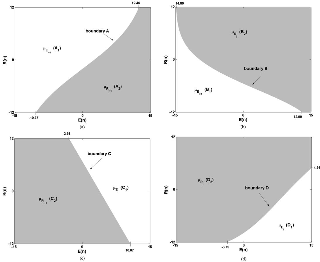
Fig. 3. Input space divisions for each of the four rules of the fuzzy controller with the input fuzzy sets shown in Fig. 2. Fig. 3(a)–(d) correspond to Rules 1–4, respectively.
