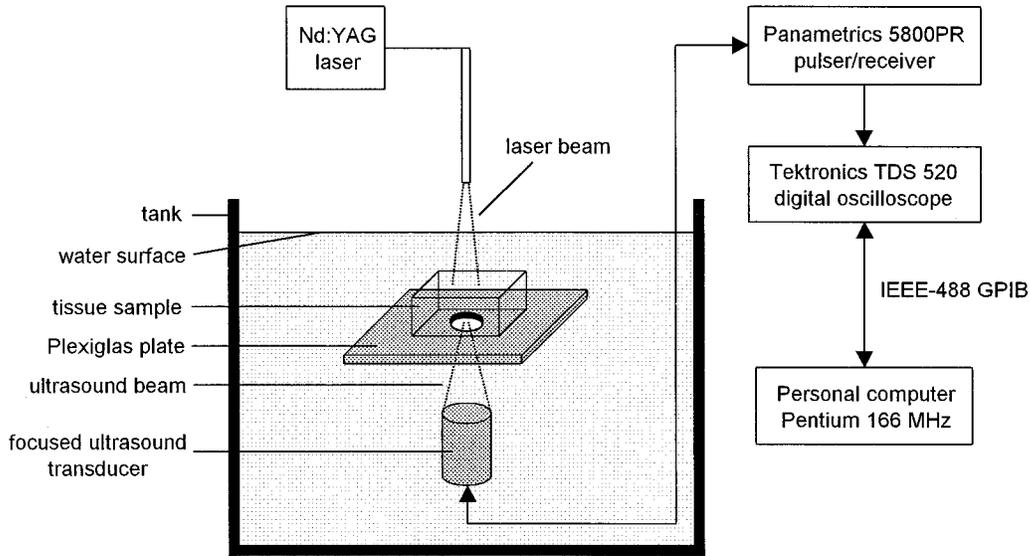
Fig. 1. Experimental setup and data acquisition system.
