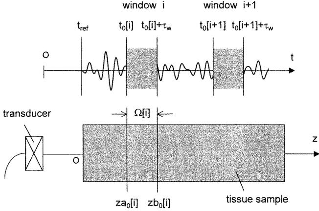
Fig. 2. Coordinate systems used throughout this paper and notations used in (1) and (2).
