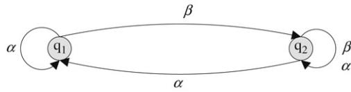
Fig. 2. The converted non-probabilistic and nondeterministic discrete event system from Fig. 1.
