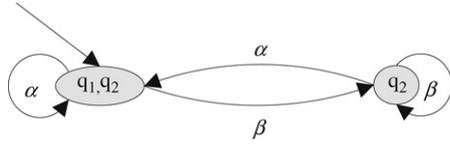
Fig. 3. The observer of the nondeterministic discrete event system in Fig. 2.
