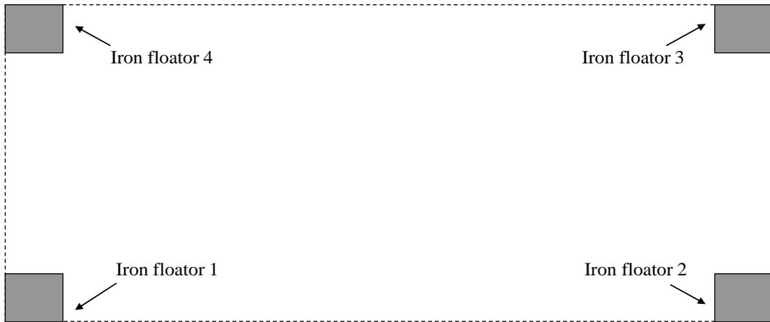
Fig. 2. Aerial view of the four equal-size iron floaters that are aligned horizontally and vertically. An electromagnetic actuator is placed above each floater (not shown here; see Fig. 1 for actuators 1 and 2)
