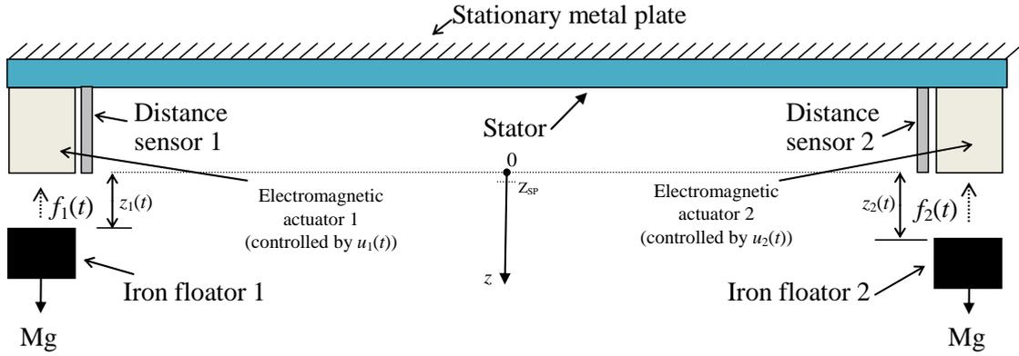
Fig. 1. Cross-section view of the simplified magnetic suspension system.
